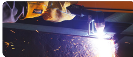
Manuelles Schneiden | Manual cutting
